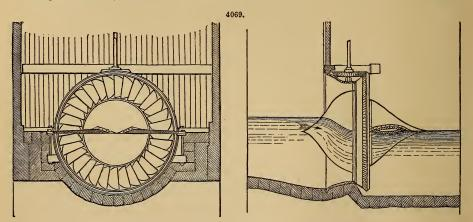
perpendicular to the direction of the water. This kind of turbine has no sluice; the volume of water which it expends increases in proportion as the fall diminishes, and diminishes, on the contrary, in proportion as the fall increases. We think it might be very advantageously applied to our large streams, in conjunction with the large turbine-wheel described above.
